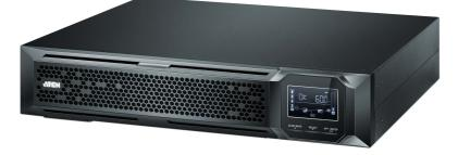
The ATEN Professional Online UPS is an exceptional and innovative electrical apparatus that provides emergency power to a load when the input power source, or the main one, fails. The basic technology of an online UPS is the same as in a standby or line-interactive UPS, however, the ATEN Professional Online UPS provides a much greater current of AC-to-DC battery-charger / rectifier where the rectifier and inverter are designed to run continuously with improved cooling systems.
