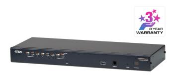
The KH1508A KVM switches are control units that allow IT administrators to access and control multiple computers from a single PS/2 or USB KVM console (keyboard, monitor, and mouse). Operators can take control of up to 8 computers. By daisy chaining up to 31 additional switches, as many as 256 computers can be controlled from the original KVM console.
