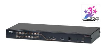
The KH2516A KVM switch is a control unit that allows IT administrators to access and control multiple computers from two PS/2 or USB KVM consoles (two bus). Operators working at up to two consoles can independently and simultaneously take control of up to 16 computers. By daisy chaining up to 15 additional switches, as many as 256 computers can be controlled from the original KVM consoles.
