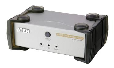
The CS231 is a powerful, micro-processor controlled computer sharing device. It is a multi-user, single-tasking device that enables two users to share the use of a single computer - each from their own consoles (monitor, keyboard, and mouse). The CS231 supports USB consoles and both PS/2 and USB computers
