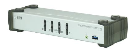
The ATEN CS1914 4-Port USB 3.0 DisplayPort KVMP<sup>TM</sup> Switch provides the latest innovations in desktop KVM switching technology to meet the increasing demand of higher video quality and file transfer rates on modern computers. The CS1914 provides superior resolutions up to 3840 x 2160 @ 30 Hz, a SuperSpeed USB 3.1 Gen 1 hub with 5 Gbps transfer rates and enhanced user-friendly operations.
