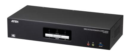
The ATEN CS1942ATC 2-Port USB 3.0 4K DisplayPort Dual Display KVMPTM Switch for ATC is tailor-made for Air Traffic Control scenarios. It supports 2Kx2K resolution, making it perfect for radar monitoring, and also enables constant monitoring of flight information and mission-critical processes. Incorporating dual display capability, users can enjoy a wider screen and easy switch between the two DisplayPort systems
