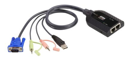
The KA7178 KVM Adapter Cable connects the KVM switch to the video, USB and audio ports of the target computer. In addition to Virtual Media support, it provides two Cat 5e/6 connectors, allowing a computer to connect to two ALTUSEN Matrix KVM switches. This allows consoles on different switches access to the same computer.
