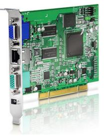
The IP8000 PCI Card combines remote "over-IP" BIOS-level access, power and virtual media functionality. This makes it a perfect solution to manage remote installations such as Kiosks, POS and ATM's. Additionally it provides IP capability to non-IP devices (Servers, KVM, etc...).
