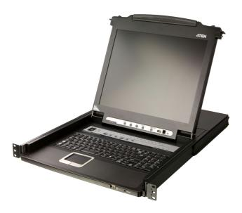
The CL5716 Slideaway – LCD KVM Switch series is a control unit that allows access to multiple computers from a single PS/2 or USB KVM (keyboard, video, and mouse) console. A single CL5716 can control up to 8 or 16 computers. As many as 31 additional KVM switches can be daisy-chained to the CL5716, so that up to 512 computers can all be controlled from a single KVM console.
