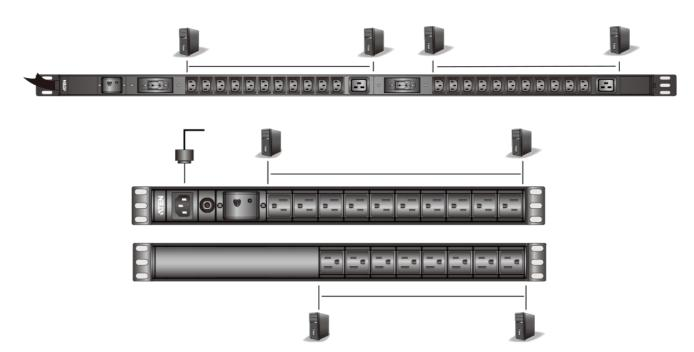
Note: (1) As there are many Basic PDUs, PE0324S (top) and PE0118S (bottom) are the respective 0U and 1U examples used here.
