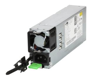
The VM3200 can be equipped with dual power modules to ensure that the system is always working. The power modules are hot-pluggable and can be easily replaced without shutting down the system. The VM3200 has two power slots that can connect to two different power supplies. If the primary power fails, the secondary power supply will automatically take over. ATEN ensures that your investment is well protected while delivering outstanding performance.
