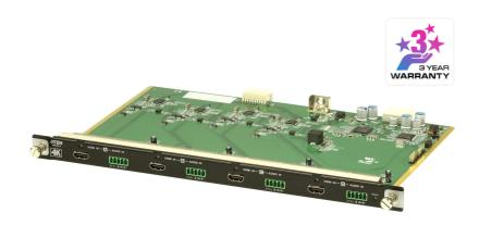
The VM7814 is a 4K HDMI input board that works with an ATEN Modular Matrix Switch to offer an easy way to route 4 HDMI sources to 4 displays. In addition to the HDMI interface that carries digital A/V signals, the VM7814 is equipped with 4 stereo audio input ports that allow stereo audio embedding.
