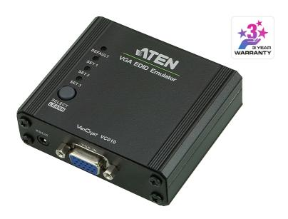
The ATEN VC010 is a VGA EDID Emulator, which is designed to emulate and store the EDID of a video display, providing constant and reliable EDID data for the a VGA source device to efficiently optimize video resolution.
