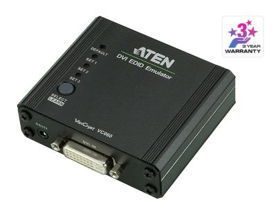
The ATEN VC060 is a DVI EDID Emulator, which is designed to emulate and store the EDID of a video display, providing constant and reliable EDID data for the a DVI source device to efficiently optimize video resolution.
