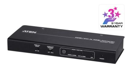
ATEN VC881 is a high-quality HDMI/DVI to HDMI converter with audio de-embedding function. Input a DVI signal and it converts the signal to HDMI signal or input an HDMI signal and it extracts the HDMI audio signal. Advanced video support provides a better-defined connection with video resolutions up to 4K and complies with HDCP 1.4.
