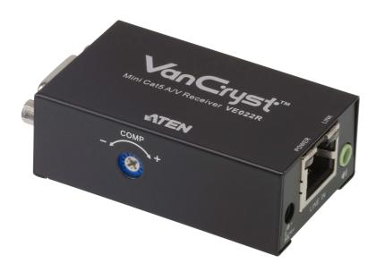
The VE022R Mini Cat 5 A/V Receiver connects with a <u>VE022</u>T to extend signals up to 150m from the source using a Cat 5e cable. With hot-plugging support, you can quickly add or remove the VE022R receiver connected to the display device without having to power down any of the devices. The <u>VE022</u> Mini Cat 5 A/V Extender is a compact, convenient and economical addition to your video/audio setup.
