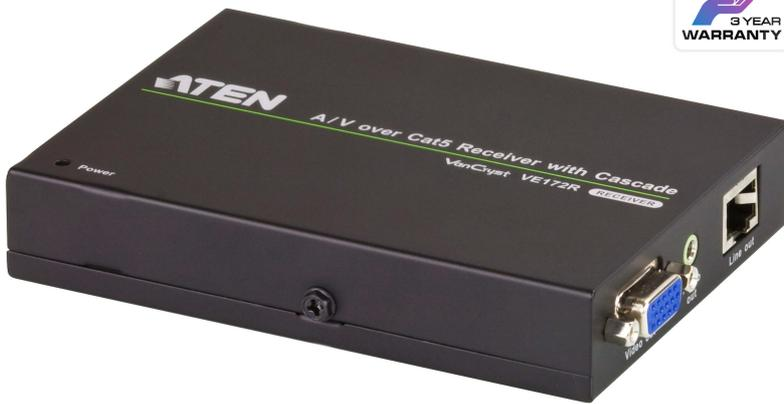
VE172R A/V Over Cat 5 Receiver is compatible with ATEN MDS Standard Plus Solution ([VS1204T/VS1208T](#), [VE170T/VE170R/VE170RQ](#)). It can cascade up to 10 levels make long distance transmissions up to 150m.
