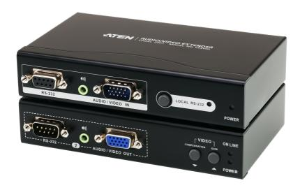
The VE200 Audio/Video Extender System allows you to extend the distance between the computer system unit and the display monitor by up to 200m/500ft for video resolutions of 1280x1024 @ 60Hz. It accomplishes this by means of a local transmitting unit (VE200L), and a remote receiving unit (VE200R), connected by Cat 5e twisted pair cable.
