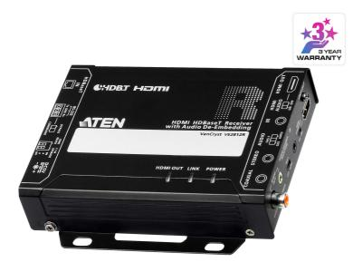
The VE2812R is a high-quality HDMI HDBaseT Receiver featuring audio de-embedding function. Powered by HDBaseT<sup>TM</sup> technology, the VE2812R can receive 4K HDMI signals up to 100 m over a single Cat 5e/6/6a or ATEN 2L-2910 Cat 6 cable. With HDBaseT Long Reach Mode enabled, it can deliver HDMI signals up to a maximum range of 150 meters @ 1080p.
