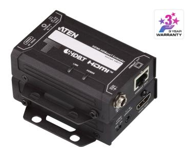
• The ATEN VE811 HDMI HDBaseT Extender guarantees the optimum 4K HDMI signal transmission across up to100 m via a single Cat 5e/6/6a or ATEN 2L-2910 Cat 6 cable. In addition, with the support for Long Reach Mode, it extends HDMI signals @ 1080p up to 150 m via a single Cat 5e/6 cable. The VE811 meets HDMI specification features including 3D, Deep Color, HD lossless audio formats and CEC pass-through. Plus, it supports Dolby Digital 5.1 and DTS HD audio.
