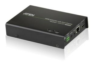
Place your HDMI displays up to 100 meters away from your HDMI source devices with the VE814R HDMI Receiver over single Cat 5 with Dual Display. Connecting to the <u>VE814T</u> transmitter via affordable and easily available Cat 5e/6 cable, your media can be streamed to up to three HDMI displays – dual displays connected to the receiver and another to the transmitter.
