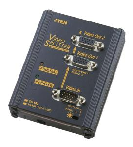
VS102 video splitters provides video input signals to 2 video outputs each at 250 MHz after duplication. Users can boost video signals from the video gain knob within a transfer range up to 65m.
