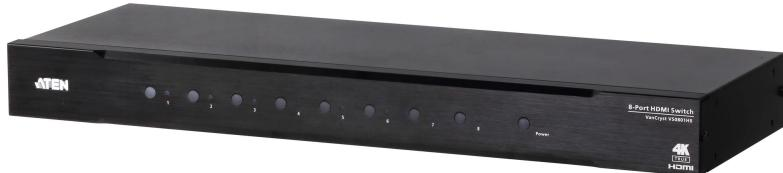
The ATEN VS0801HB is designed for applications that require the routing of 8 sources to one compatible display device. It supports video resolutions up to True 4K (4096 x 2160 @ 60Hz 4:4:4), data rates up to 18 Gbps, 3D, Deep Color up to 12-bit, and HD lossless audio formats. The VS0801HB features Auto Switching modes for auto port selection. Multiple convenient control options include front panel pushbuttons, bi-directional RS-232, IR, and auto switch, allowing for easy integration.
