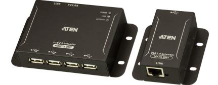
The UCE3250 4-port USB 2.0 Cat 5 Extender is a two-unit device that serves as a USB hub and a USB extender. The UCE3250 unit can connect as many as 4 USB peripherals from up to 50 meters away from your computer over an Ethernet cable.
