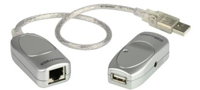
UCE60 lets you locate your USB device or hub up to 60m (198 ft) from your computer, overcoming the typical USB cable limitation. It conditions the USB signals to communicate up to 60m using low-cost Ethernet cable.
