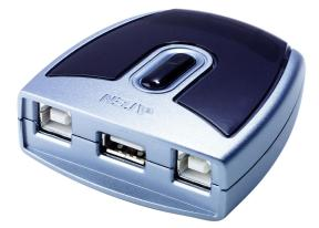
US221 allows 2 computers to share the same USB peripheral under the foundation of one-at-a-time. Users can switch the computer controlling the peripheral from the simple hotkeys or buttons on the front panel or the control software on Windows. It is ideal for SOHO environments. 20050223153137004.jpg
