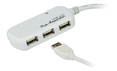
The UE2120H allows users to extend the distance between a computer and USB device(s) up to 12 meters via the active extender hub. USB signals transmitted through these cables maintain optimal signal integrity and meet USB 2.0 standards. Up to 4 extender cables (<u>UE2120</u>) and 1 Extender Hub (UE2120H) can be chained together, so that cable distance is increased by up to 60 meters.
