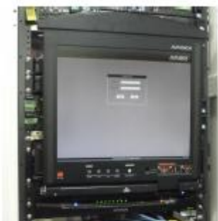
Monitoring the status on the LCD module while the keyboard module of LCD console KL1100 slides back to the rack. KL1100 is installed on the top and the device below is the KN4124v KVM Over the NET.
