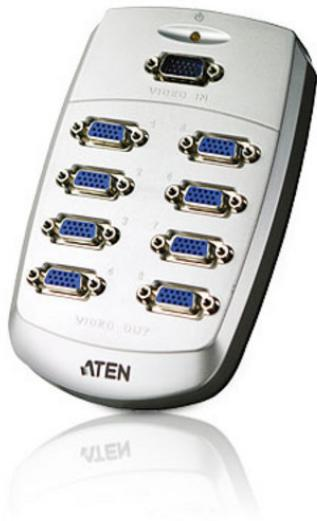
The VS88 Video Splitter duplicates the video signal from an input source (i.e. a computer) and route it to up to 8 display devices (monitors, projectors, etc.). However, they go beyond being merely duplicators, in that they also enhance the video signals over distances up to 30 meters. Furthermore, they can be cascaded three levels to additional ATEN video splitters to support many numerous display devices. And they mount inconspicuously on the wall or out of sight.
