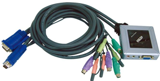
The CS62B 2-Port KVM Switch is a control unit that allows access to two computers from a single console (keyboard, monitor, and mouse). Before the development of the CS62B, the only way to control multiple computer configurations from a single console was through a complex and costly network system. Now, with the CS62B KVM Switch, you can easily access two computers in a cost effective manner.
