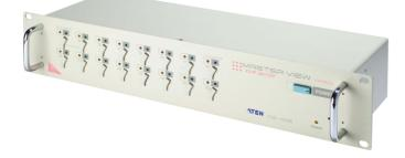
CS1016 KVM Switch is designed according to the needs of server rooms of larger scale. It uses the DB-25 interface to integrate relevant signals, reduce cable derangements, and enhances signal quality and operation efficiency. CS1016 supports OSD (On Screen Display) menu function to facilitate operators to switch between computers. It also supports microphone and amplifier functions. 2005022410196005.jpg
