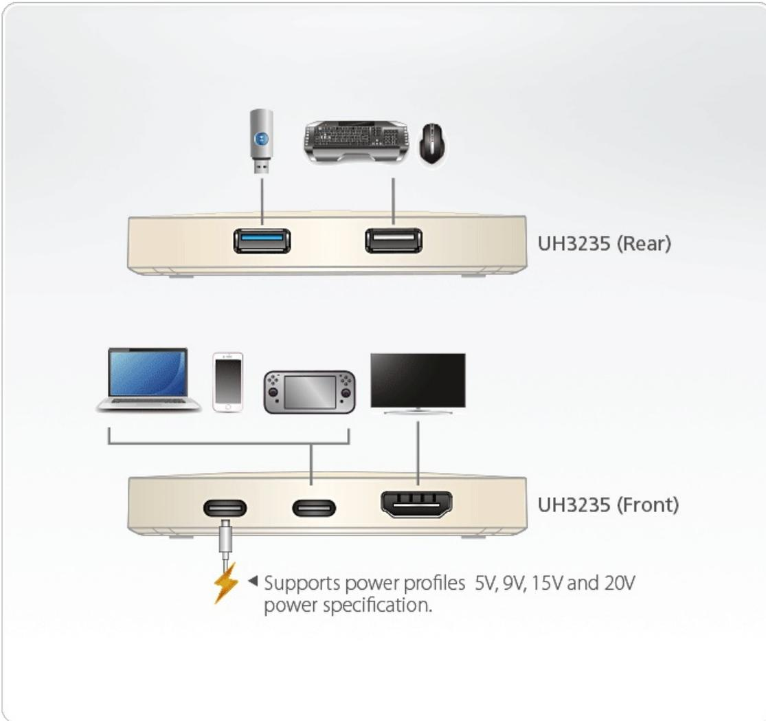
⚡ Supports power profiles 5V, 9V, 15V and 20V power specification.
