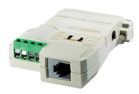
IC485S is a 2-way converter for converting RS-232 signals to and from RS-422/RS-485 signals in long-distance applications up to 1200 m (4000 ft.). It supports the connection of up to 32 hubs and features monitoring to confirm the data passing between devices.
