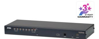
The KH1508A KVM switches are control units that allow IT administrators to access and control multiple computers from a single PS/2 or USB KVM console (keyboard, monitor, and mouse). Operators can take control of up to 8 computers. By daisy chaining up to 31 additional switches, as many as 256 computers can be controlled from the original KVM console.
