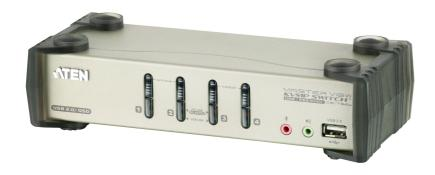
The CS1734B is 4-port KVM switch combined with a 2-port USB 2.0 hub. As a KVM switch, it allows users to access four computers from a single keyboard, monitor, and mouse console. There are four methods to obtain instant access to any computer in your installation: Pushbuttons, Hotkeys, OSD, and mouse.
