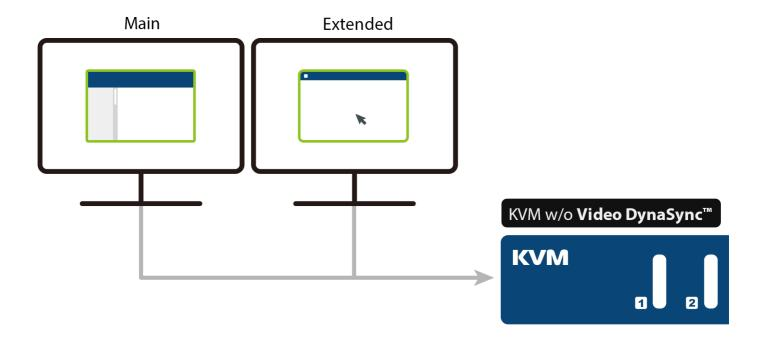
For requirements of more displays to monitor, users can daisy-chain two CS1842 for up to four displays to multitask easily and process tremendous information. Besides, a remote port selector is available for quick and streamlined port selection apart from pushbuttons, hotkeys and mouse port switching.
