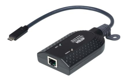
The KA7183 KVM Adapter empowers any Cat 5 KVM switch\* to connect to and manage a USB-C compatible target computer. Via just a single USB-C plug, it is able to connect a target computer while fulfilling keyboard, video, mouse, and virtual media or smart card / CAC reader functions.
