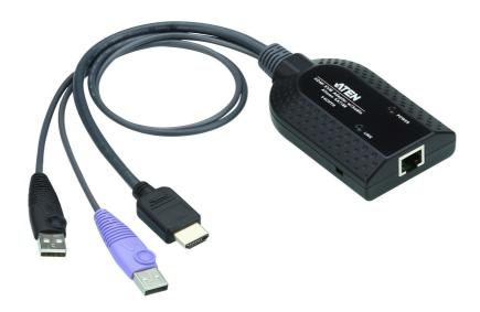
The KA7188 KVM Adapter Cable connects a KVM switch to the HDMI video and USB ports of a target computer.\* The KA7188 supports HDMI output and provides two USB plugs to connect a target computer for keyboard/mouse, Virtual Media, or Smart Card/CAC Reader functions.\*\*
