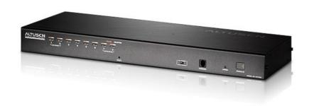
The KH1508i KVM Switche is control unit that allow access to multiple computers from a single KVM console. It uses TCP/IP for its communications protocol, it can be accessed from any computer on the Net - whether that computer is located down the hall, down the street, or half-way around the world.
