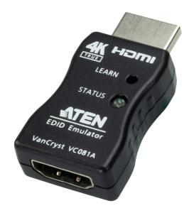
As a True 4K HDMI EDID Emulator Adapter , the VC081A is designed to emulate and store one set of the EDID from the connected display while facilitating 4K video transmission. By learning the EDID from the HDMI display and relaying it to the video source, the VC081A helps to eliminate video communication problems that occur due to the EDID data synchronization failure between the HDMI video source and the connected display.
