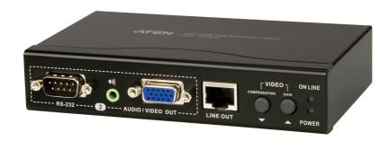
The VB552 VGA Over Cat 5 Repeater +Audio is an audio/video signal extension device which is compatible with ATEN Cat 5 Audio/Video splitters. The VB552 extends the audio/video transmission range an extra 150m over Cat 5e (or higher) cables. The use of an additional repeater means the audio/video signals can be transmitted over even longer distances, up to 450m.
