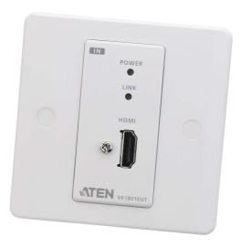
ATEN VE1801EUT is a transmitter designed to reliably send 4K signals up to 40 m over a single Cat 5e/6/6a or ATEN <u>2L-2910</u> Cat 6 cable. With EU Wall Plate design, the VE1801EUT can be conveniently mounted in a one-gang junction box. For HDMI signal transmission, it supports 3D, Deep Color, and embedded HD lossless audio formats.
