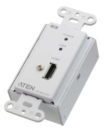
ATEN VE1801UST is a transmitter designed to reliably send 4K signals up to 40 m over a single Cat 5e/6/6a or ATEN <u>2L-2910</u> Cat 6 cable. With US Wall Plate design, the VE1801UST can be conveniently mounted in a one-gang junction box. For HDMI signal transmission, it supports 3D, Deep Color, and embedded HD lossless audio formats.
