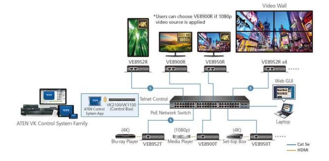
\*Note: VE8952 supports PoE and can be installed in combination with PoE network switches to reduce power cabling and additional power outlets. Before choosing the Network switch and installation, please refer to the Implementation Guide
