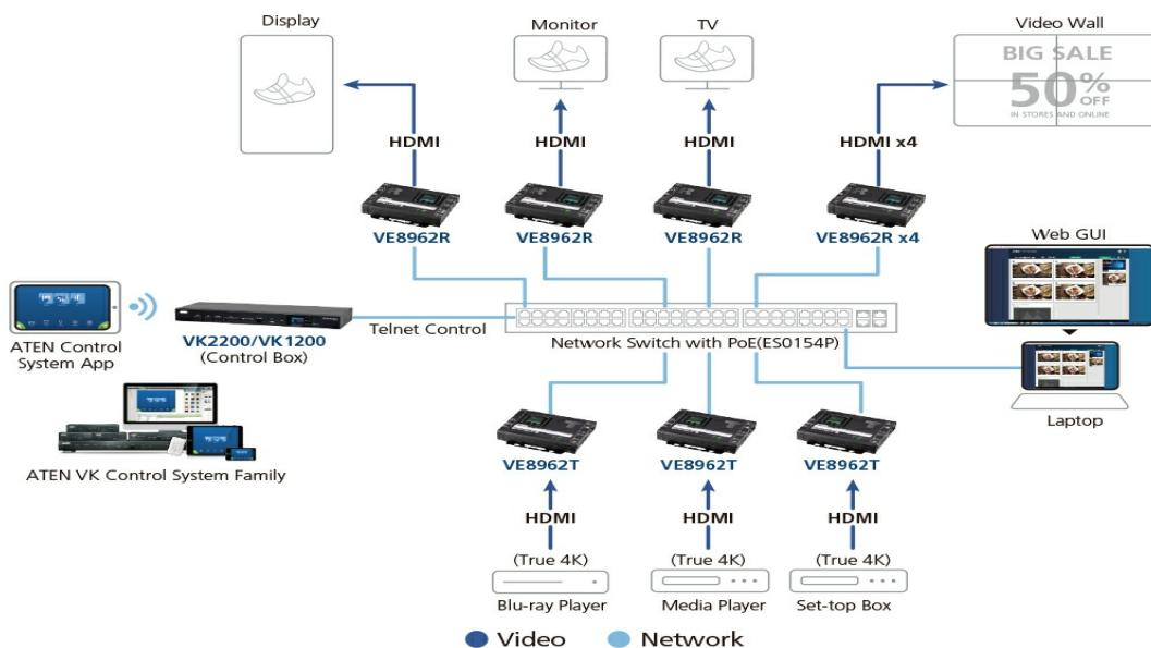
Note: VE8962 supports PoE and can be installed in combination with PoE network switches to reduce power cabling and additional power outlets. Before choosing the Network switch and installation, please refer to the Implementation Guide.
