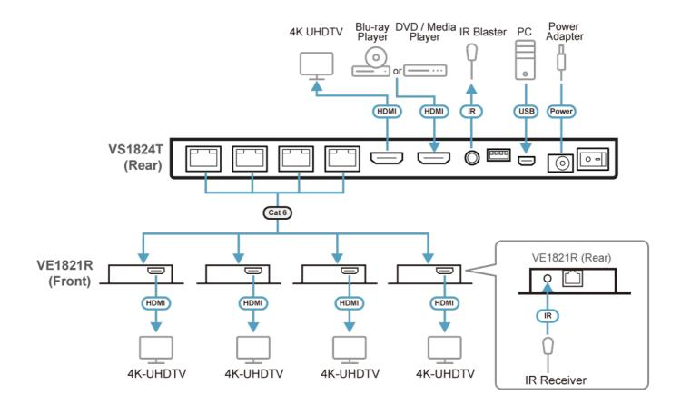
Note: Only connect VS1824T with VE1821R. Connecting VS1824T with other receiver models or third-party receivers may cause physical damage to the receiver.
