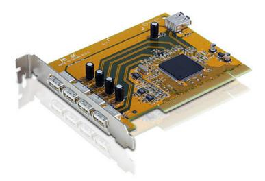
IC250U is a PCI card with 5 USB ports. It supports hot plug and PnP.
