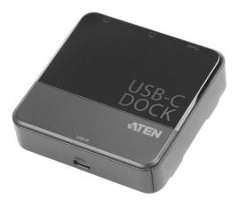
The ATEN UH3233 is a USB-C Dual-HDMI Mini Dock which transforms your USB-C device to a dual monitor workstation. It's compliant with the latest USB 3.2 Type-C specifications and supports dual display mode. The UH3233 can route video from the source device to two HDMI monitors, splitting the video transmission for a dual-view display via a single cable while maintaining a high quality resolution up to 1080p.
