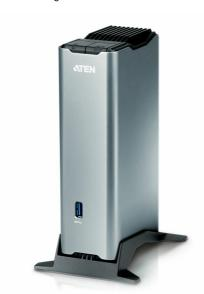
The US7220 Thunderbolt 2 KVM Docking Station is a dual-computer KVM docking station for your workspace. You can share Thunderbolt devices, a dual-monitor setup and USB peripherals through a single cable, directly to two computers.
