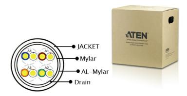
The 2L-2901 Shielded Digital Video Extension Cable is a twisted pair shielded with conductive metal film. The cable utilizes copper wires, which are widely used for data transmission. Its outer metal layer protects signal transmissions from electromagnetic interference and reduces the impact caused by electrical noise. The 2L-2901 can support long distance connections while safeguarding transmission quality.
